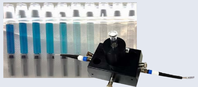
Figure 1: Syringes containing methylene blue solutions at different concentrations and the syringe-holder allowing repeatable measurements.
